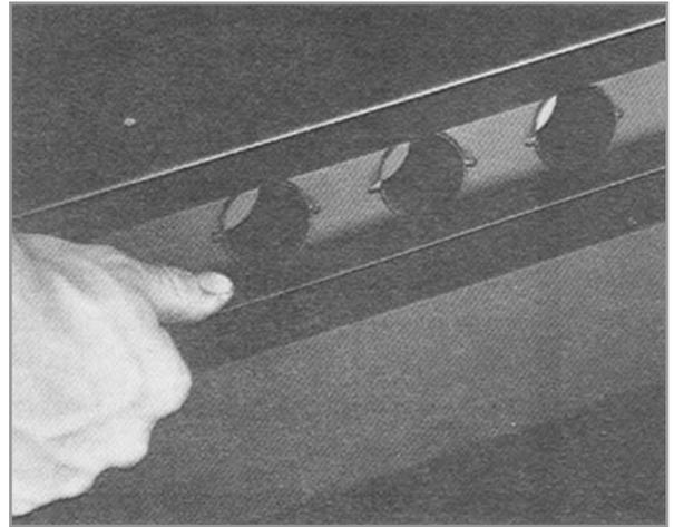
**SPIGOT RESTRICTOR :** The spigot restrictor is supplied fitted to the fire as a stitch bent plate on the flue outlet. If installing the fire into a class 1 or a good class 2 flue, bend up into position in the flue outlet of the fire.
