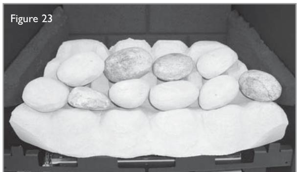
5. Place the rear row of five pebbles, making sure that the flat sides are firmly against the brick panel and side cheeks as shown. The pebbles must not be crammed together, or inserted into the holes in the matrix. A well laid out, generously spaced pebble layout will give the best results.
