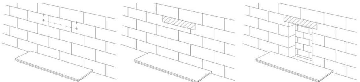
The non-combustible hearth may now be put in place. Again this should not bridge the cavity where it projects into the wall space. Finally install the fireplace or fire surround and back panel/marble to its finished location.
