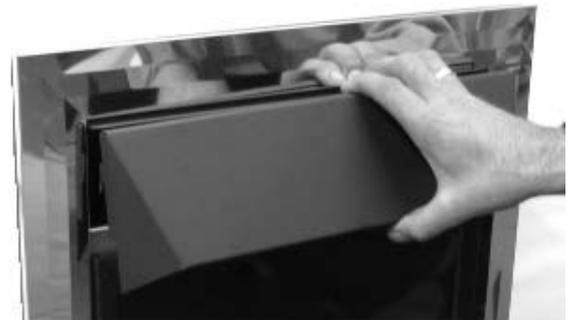
Fit the convector hood to the firebox by engaging the two mounting hooks into the relevant slots in the firebox. The hood should be pressed inwards and downwards to secure into position.
