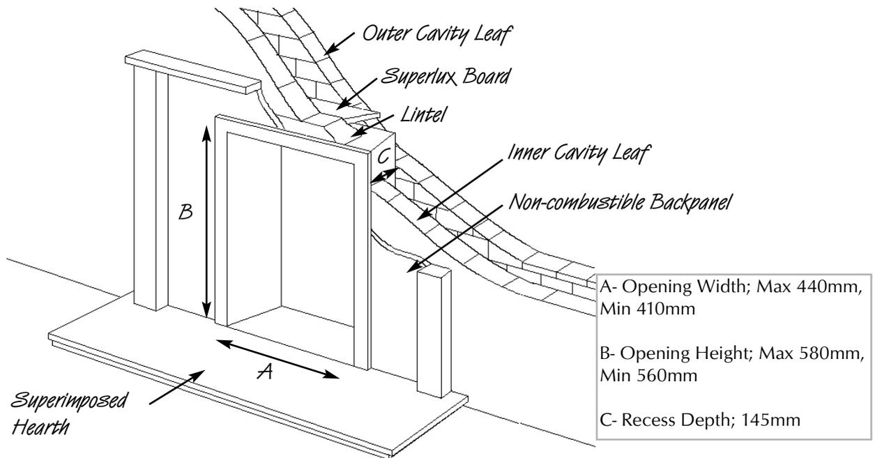
Check the cavity insulation type (if applicable). If cavity insulation is of a loose fill variety, take precautions to prevent excessive loss of material when the inner leaf is opened up by packing the cavity firmly with a minimum 50mm of rockwool or glass fibre. This will hold back any loose material now or in the future.
