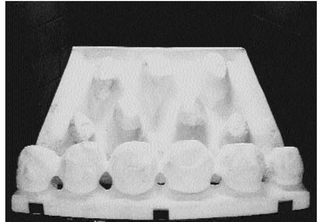
2. Open the bag of 16 ceramic pebbles. All of these pebbles are the same. Take five pebbles and place them as shown. Care should be taken to ensure that the pebbles bridge the gap between the front strip and the four supports at the front of the matrix. Care should also be taken not to push the pebbles right down between the supports, as this can affect the flame picture when the appliance is running.
