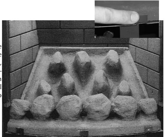
3. Open the bag of 16 moulded coals. All of the coals are the same. Take five coals and place them as shown. Care should be taken to ensure that the coals bridge the gap between the front coal and the four coal supports at the front of the matrix. Care should also be taken not to push the coals right down between the coal supports, as this can detract from the flame picture when the appliance is running.
