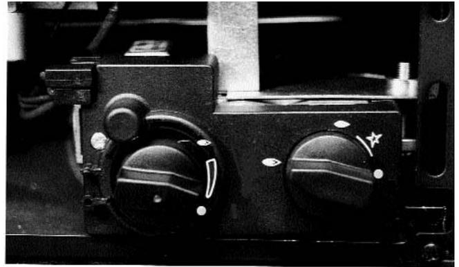
If the pilot is extinguished during use of the fire, you must wait three minutes before repeating the ignition procedure.
